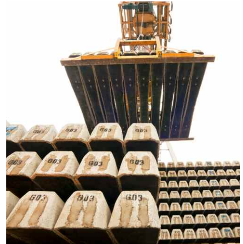
Installation of sleepers at the RailOne plant
